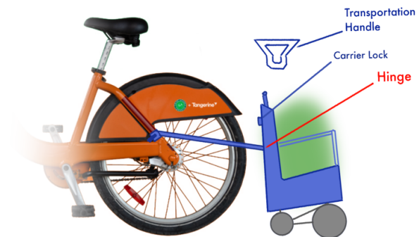
Figure 9: Back axle trailer design
