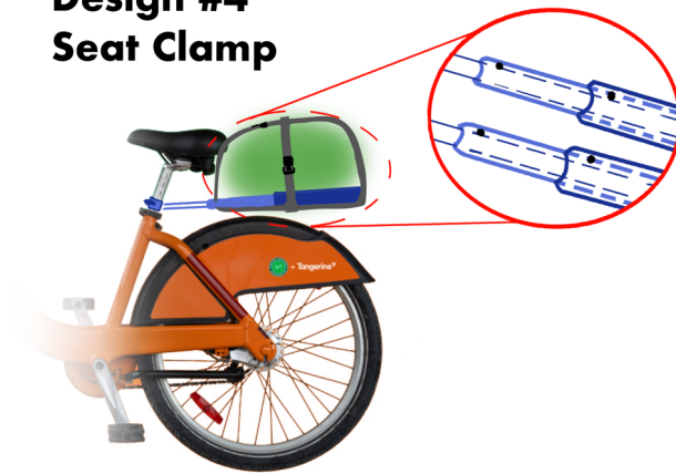
Figure 10: Candidate design #4. A platform for the backpack clamped onto the seat post.
