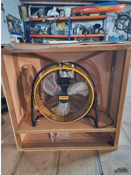
Section 3 of the wind tunnel (ventilator)
