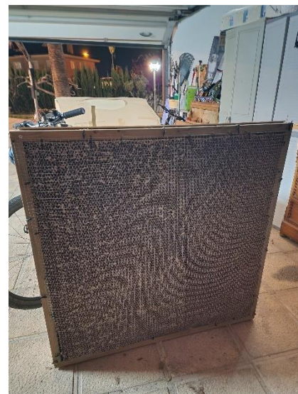
Honeycomb mesh in section 1 of the tunnel
