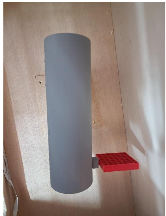
Figure T12: Grid fin attached to the model rocket
